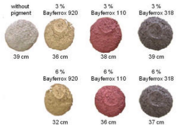
Slump (water/cement ratio 0.56)
